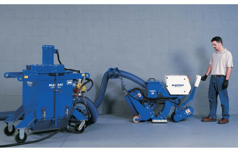
Blastrac<sup>®</sup> shot blasting is a cost-effective and environmentally friendly method for preparing concrete and steel surfaces. It is the surface preparation method recommended by most coating manufacturers.
